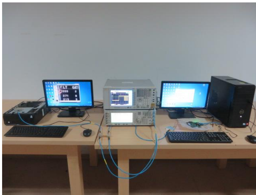
DFS Test Set-up Photo for Master Device - Set-up A
